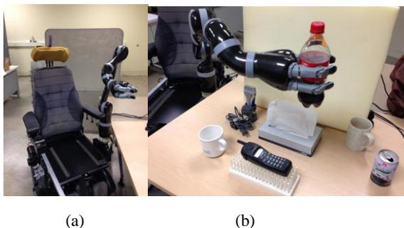
Fig. 5. (a) JACO robotic arm (b) Object manipulation.
