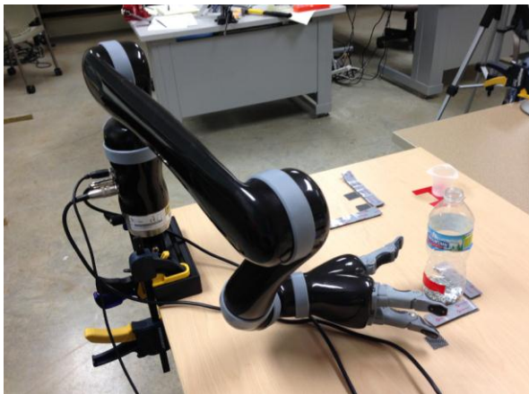
Fig. 1. JACO robotic arm ready to grasp a water bottle. It can also be mounted to a wheelchair.
