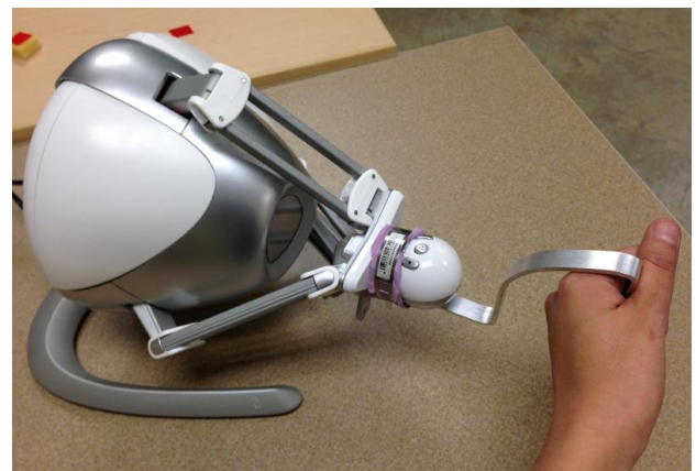
Fig. 3. 3D joystick with adapted handle for quadriplegic users.
