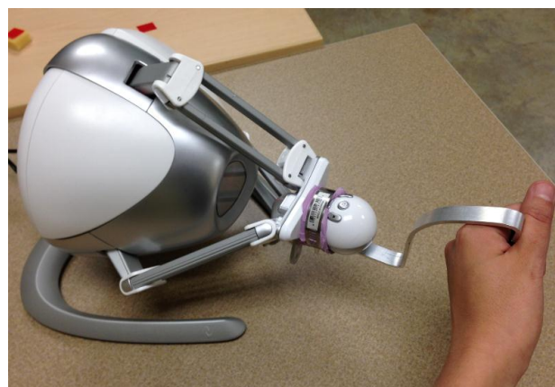
Fig. 3. 3D joystick with adapted handle for quadriplegic users.
