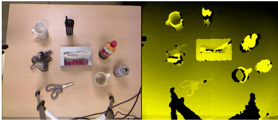
Fig. 3. (a) Color frame of test objects (b) Depth frame of test objects.
