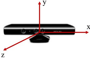
Figure 4. Kinect coordinate system
