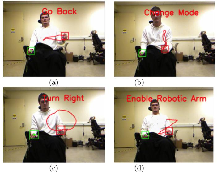
Fig. 15 Gesture mapping for robotic control
